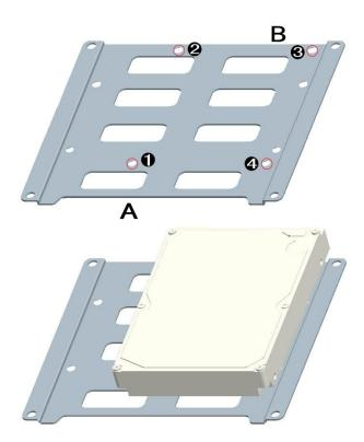
2. Install 2.5" HDD/SSD onto HDD bracket
