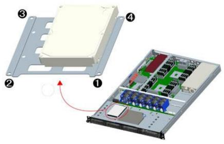
3. Install HDD bracket onto chassis
