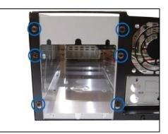
2.Secure the power supply on both side of chassis
