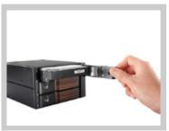
3) Remove HDD from the cage.
