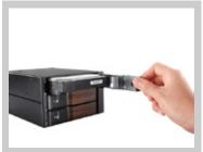
3) Remove HDD from the cage.
