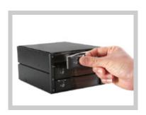
2) Slide in HDD halfway into the cage and close the handle until the lever clicks. The HDD is now connected to the backplane.
