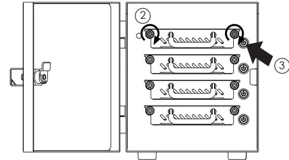
2. Tighten two hand screws to secure HDD tray
