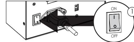
1. Make sure power switch in the back of chassis is in ON position
