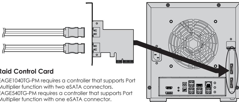
\*please make sure all the cable connectors are secured (locked) properly.
