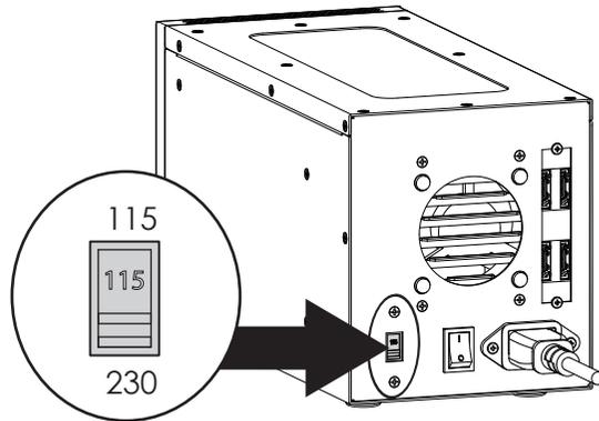
1. Switch to right voltage setting before turning on power switch
