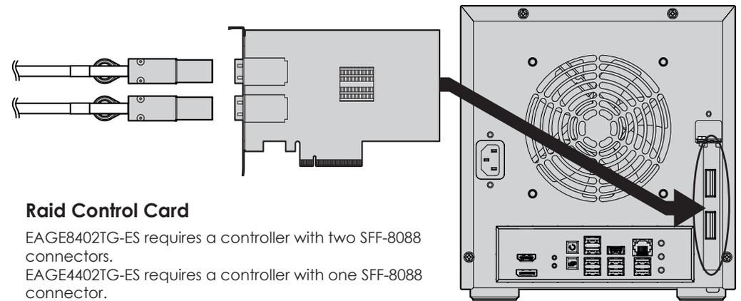
\*please make sure all the cable connectors are secured (locked) properly.
