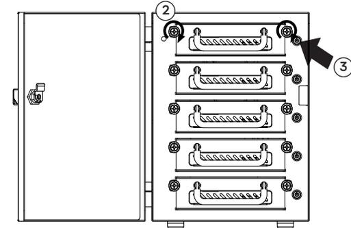
2. Tighten two hand screws to secure HDD tray
