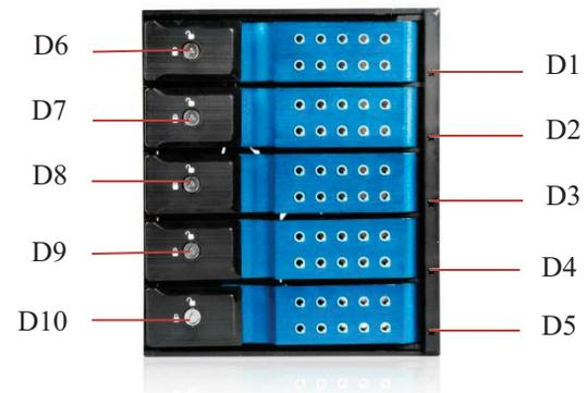
**D-1 ~ D-5:** HDD LED. Power On, LED indicates Blue. Purple blinking for HDD access.
