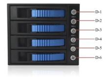
**D-1**: Reset Switch & Overheat LED. Power On: LED indicates Blue. Overheat (default 55° C): LED indicate Red and buzzer alarms. Press the Reset Switch (D-1) to stop the alarm for 3 minutes.
