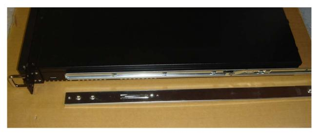
b. Mount the L Shaped Bracket onto the outer channel. Make sure the end of the bracket could touch the chassis' handle.
