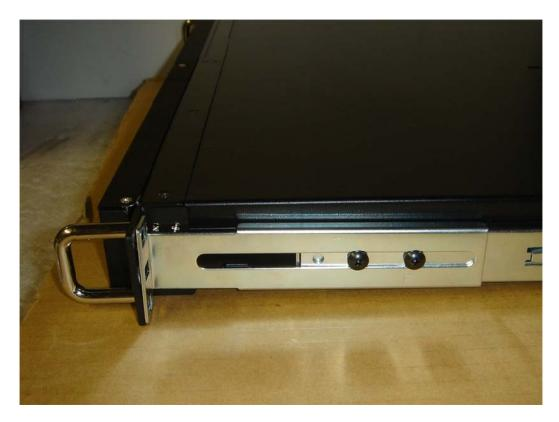
c. Mount another L Shaped Bracket to the other side of the channel. Adjust the position according to the cabinet's length. By doing this, the chassis' handle should touch the cabinet very well.
