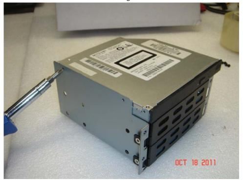
4. Mount the whole HDD cage with the slim optical drive back to the chassis
