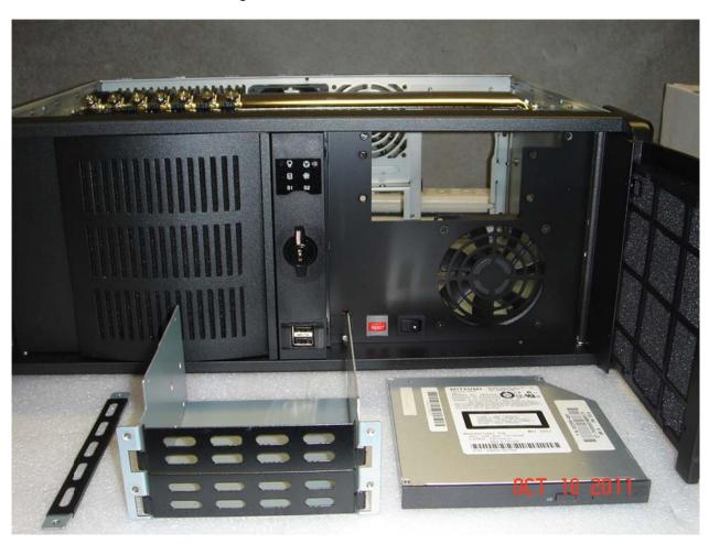
3. Mount the 5.25" Slim Drive on the HDD cage
