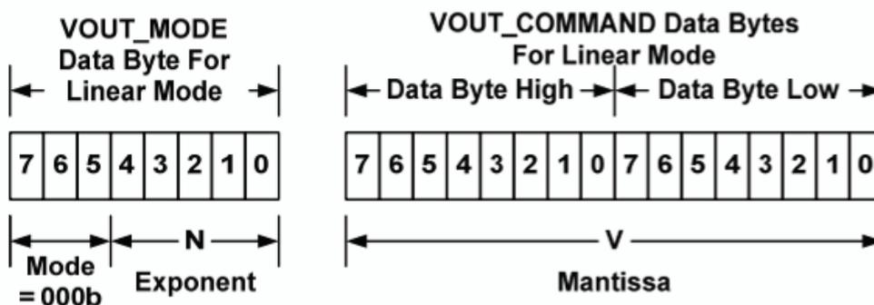
The Voltage, in volts, is calculated from the equation:
