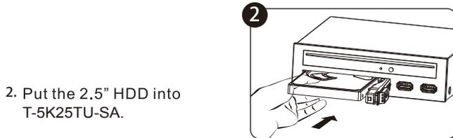
2. Put the 2.5" HDD into T-5K25TU-SA.
