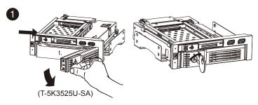
1. Release the door puller to eject the front door panel Triangular lock unlock with the key (clockwise rotated 90 degrees), open the panel
