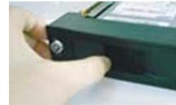
1. Pull the spring lock to open the front door.
