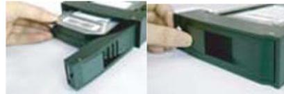
2. Place the hard drive into T5-SA with the HDD label(printed) side up and be sure the HDD connectors side is inserted
