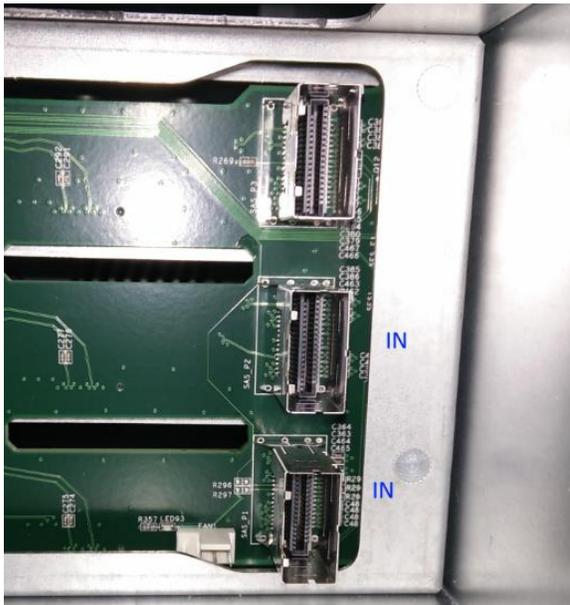
2. Connect either one of the bottom two connectors from the rear 12-bay SAS expander backplane to a controller to access all 12 hard drives.
