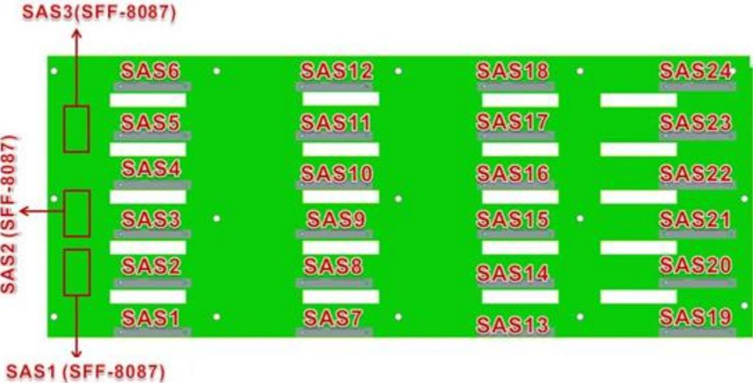
1. Only need to connect one of the three connectors from the front 24-bay SAS expander backplane to a controller to access all 24 hard drives. Try with different connectors if the controller doesn't not recognize the SAS expander backplane.
