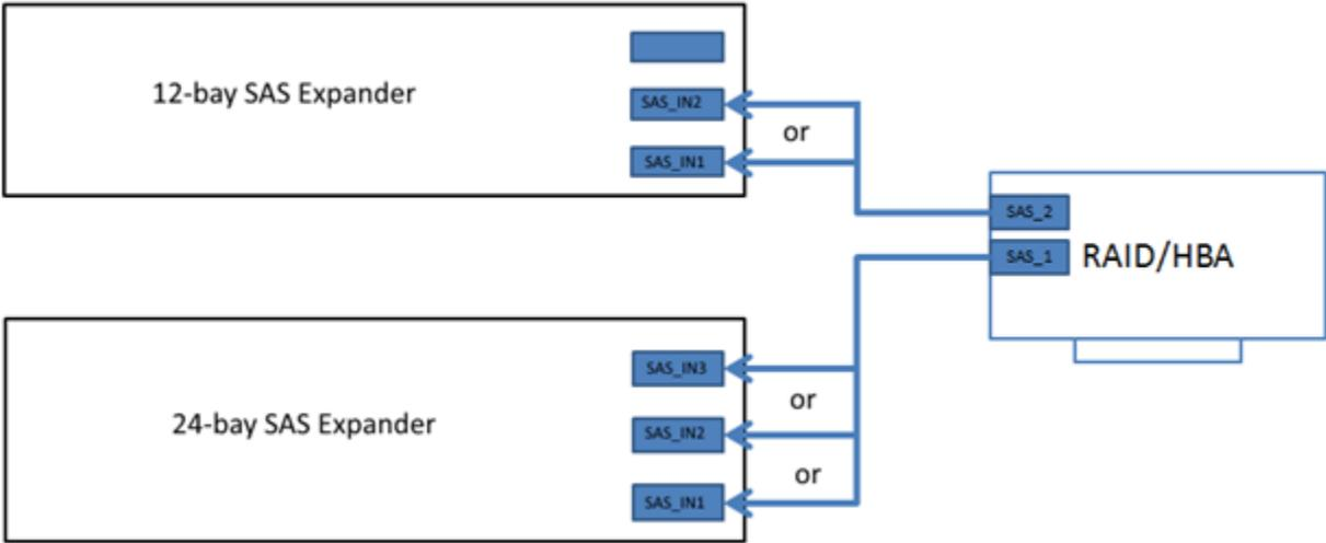
Connection Diagram of Controller and SAS Expanders
